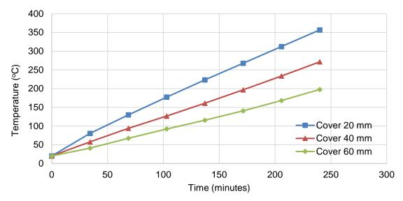
Fig. 13- Effect of changing the concrete cover thickness on thermal response of beam
