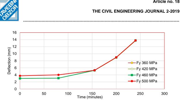
Fig. 15- Effect of changing reinforcement yield strength on structural response of beam
