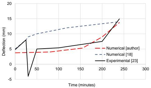
Fig. 7 - Variation of mid-span deflection with exposure time
