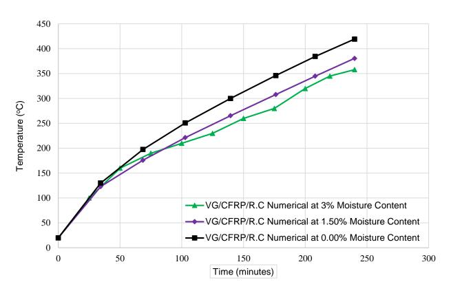
(b) Effect of moisture content on the thermal response of VG/CFRP/R.C interface
