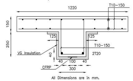
Fig. 1- Cross-section of experimentally tested T-beam [23] DOI 10.14311/CEJ.2019.02.0018
