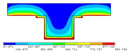
Fig.5 - Numerical predicted temperature distribution in beam cross-section (°C) after four hours
