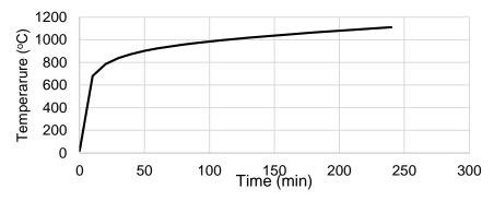
Fig. 4- Applied temperature conforming to Standard Fire Test Curve of ASTM E119
