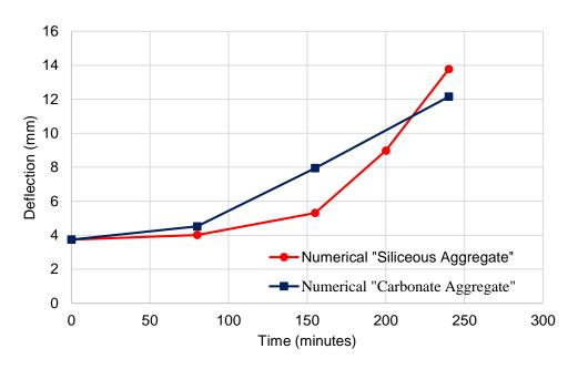
Fig. 8 - Mid-span deflection for different concrete aggregate types
