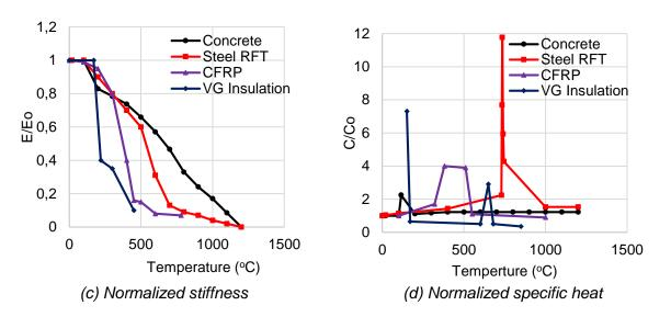
Fig. 2 - Variation of mechanical and thermal properties of materials with temperature
